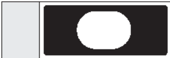
Figure 93 Standard 25 mm x 75 mm x 1 mm slide used during the manufacturing of 17 x 24 mm oblong, single well fluorescent particle slides.
